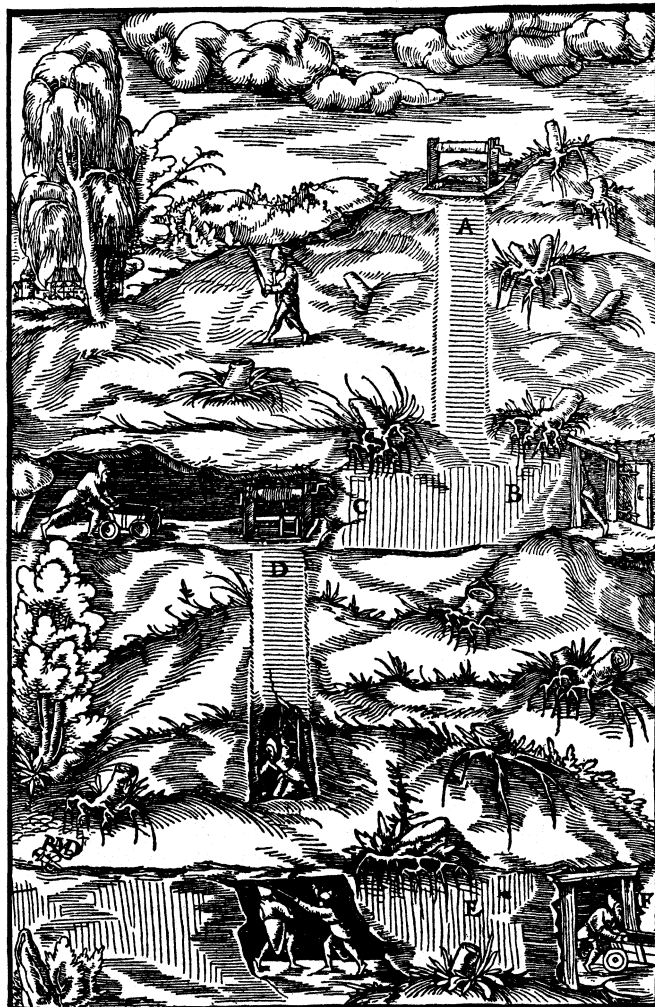
FIG. 1.—EARLY MINING METHODS IN "DE RE METALLICA" (1566) BY GEORG AGRICOLA A. Shaft. B, C, D. Drifts. E. Tunnel. F. Tunnel mouth
