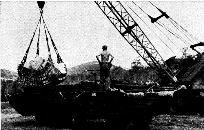
Crane hoisting load of supplies from a dukwa, or duck, a 2½-ton amphibious vehicle equipped with an engine which could drive its wheels on land or propellers in the water. The dukwa was used as a shuttle craft between supply ships and cargo dumps ashore during World War II in all theatres of operation
